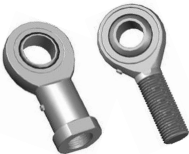
Rod ends EXPI..VW, EXPE..VW Steel/Bronze outer ring with bronze liner, with lubricating hole or nipple, with right or left-hand & male or female thread.
