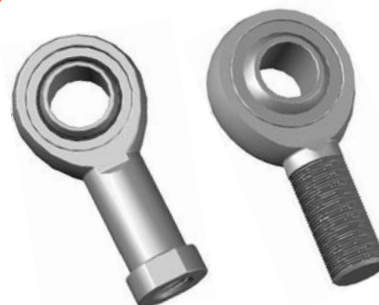
Rod ends SS EXTI..VW , SS EXTE..VW Stainless Steel/PTFE made up of a maintenance free radial spherical plain bearing and rod body, with right or left-hand & male or female thread.
