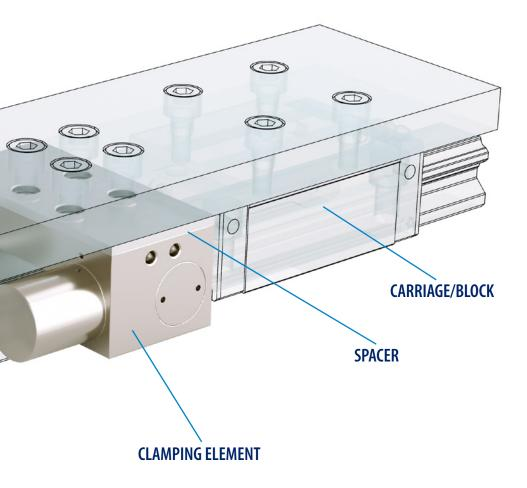
Clamping and braking elements can optionally be supplied with a "spacer" plate made in Steel, used to align the height of the element with the height of the sliding guides.
