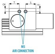
we recommend the use of compressed air hose ø 6x4 FRC##\$ SEM FRC##\$ DEM
